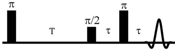
FIG. 1. IRESE pulse sequence for  $R_{1e}$  imaging.
