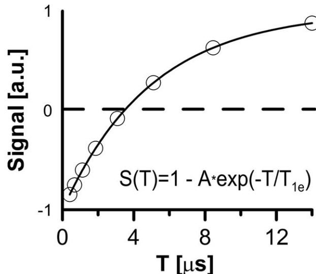
FIG. 2. Simulation of a single voxel's signal amplitude dependence on  $T$  in IRESE sequence.  $T_{1e} = 5 \mu s$  was used.
